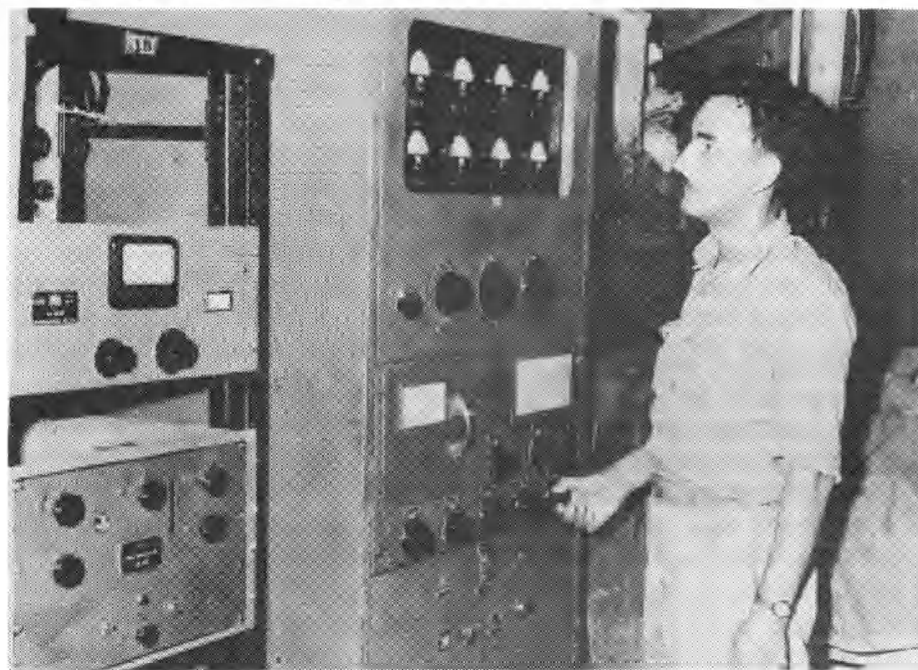
Engineer George Luckey shown with 400-watt PZ transmitter. Keying unit and frequency shift exciter in rack to the left.
